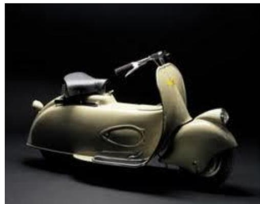
arm similar to an aircraft carriage. Finally, he designed a body that would protect the driver so that he would not get dirty or disheveled. Decades before the spread of ergonomic studies, the riding position of the Vespa was designed to let you sit comfortably and safely, not balanced dangerously as on a high-wheel motorcycle.
